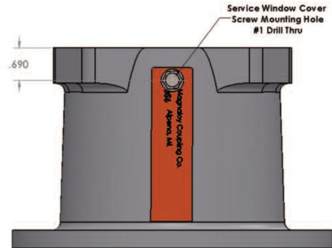
M056 Mount with New Cover installed. The Cover has been cut to length to cover the Service Window Opening. The mount has been drilled at the indicated location and the mounting screw installed.
